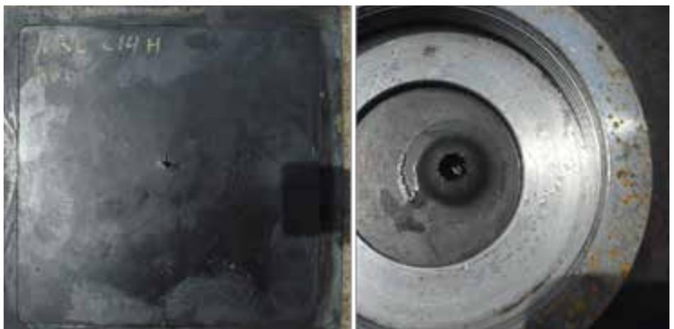
Figure 4: Elastomer Coating on Front of Steel Tank After Penetration by .50-cal. AP Round (Left); Hole in Center Has Completely Closed; Backside of Steel Vessel, With Hole Approximately 50% Larger Than Bullet Diameter (Right).
