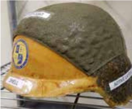
Figure 5: Advanced Combat Helmet Core With Added Layer of Resonating Elastomer Containing 33% Hollow Spheres. The Latter Have the Same Density as the Polymer, So the Helmet Weight Is Independent of Sphere Content.
