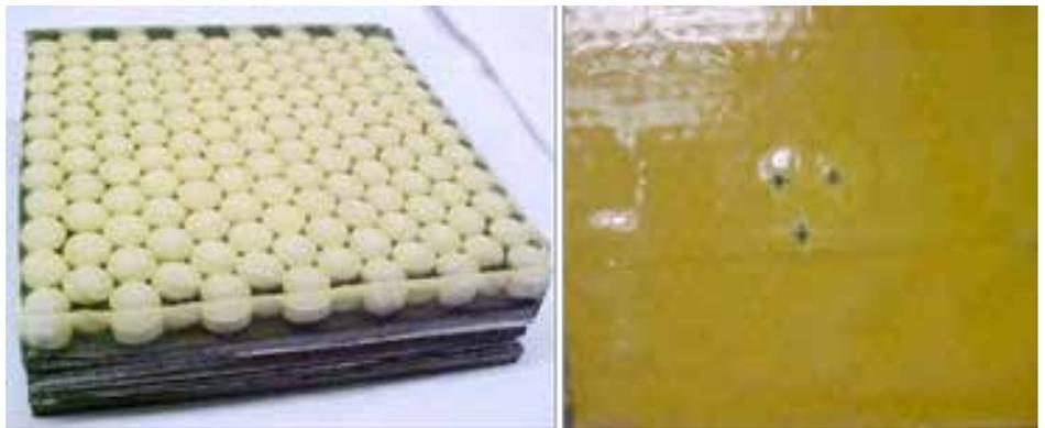
Figure 3: Ceramic Spheres Embedded in Elastomer (Left); Front-Side After Penetration by Three 0.50-cal. AP Rounds Falling Within 2-inch Circle (Stanag 4241 Bullet Impact Test), Showing Small Holes in Kevlar Top Layer (Right). The Damage Zone Is Less Than the Bullet Diameter Because the Elastomer Contains the Ceramic Granulated by the Projectile.
